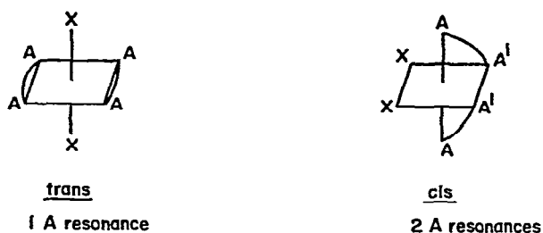
Fig. 21. The two geometrical isomers of an M(AA)_2X_2 complex illustrating the number of different resonances possible for the terminal groups of the AA ligands.
